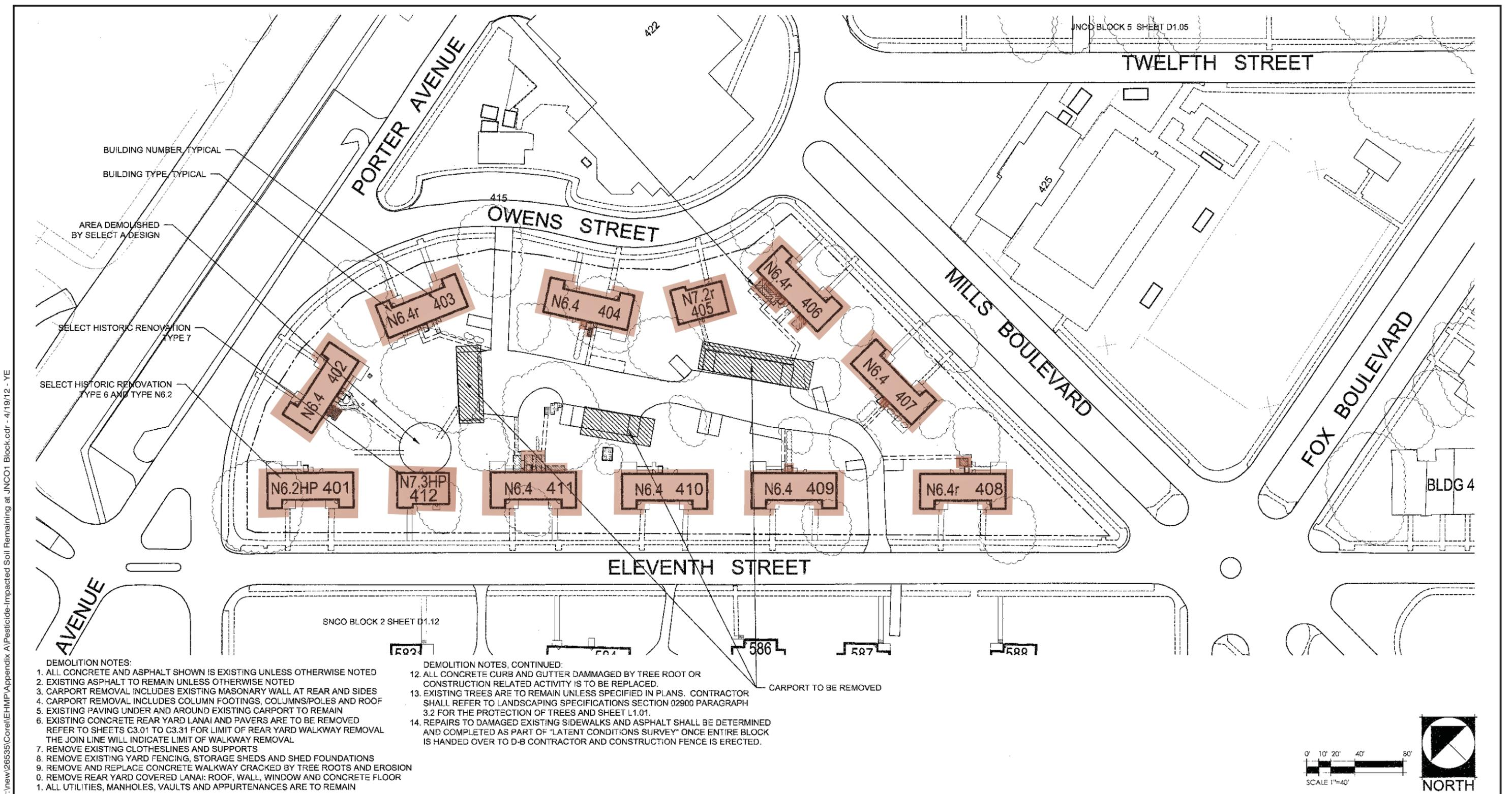
The 3 foot building zone depicted on the map is estimated. The actual 3 foot distance will be measured and marked in the in the field prior to excavation.
