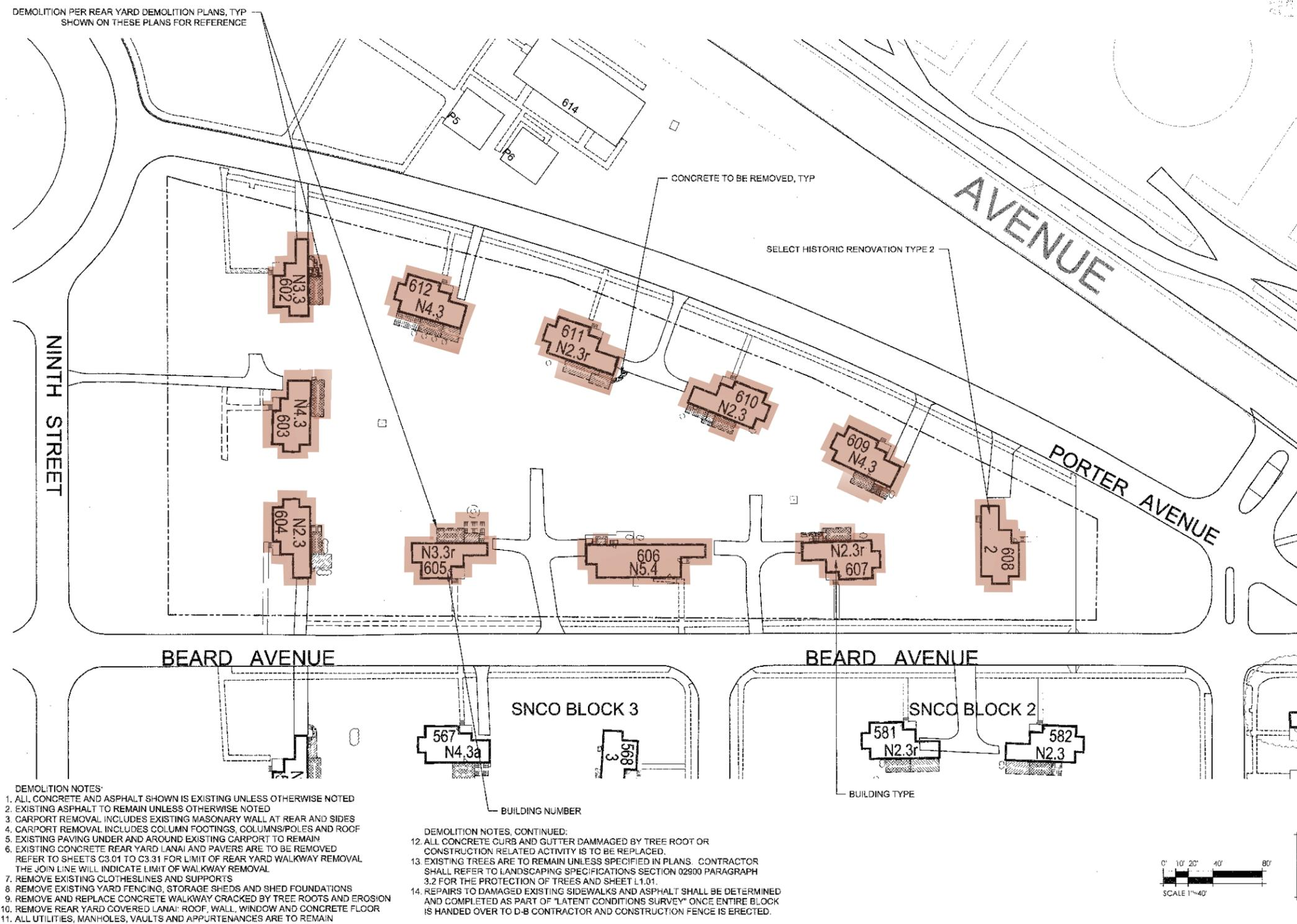
The 3 foot building zone depicted on the map is estimated. The actual 3 foot distance will be measured and marked in the in the field prior to excavation.
